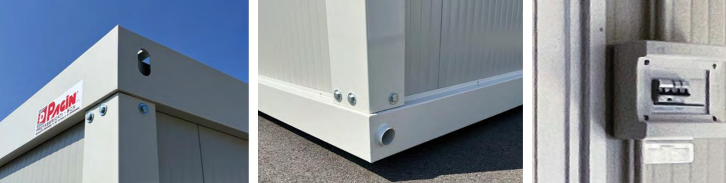
**TECHNICAL SPECIFICATIONS:** Frame with galvanized and painted 30/10 profiles. Interchangeable insulated 50 to 100 mm thick walls in PUR, smooth sheet on both sides. Insulated 50 to 100 mm thick roof in PUR + 40 mm thick reinforcement rib. 18 mm thick floor made of waterproof chipboard covered by a PVC sheet. Lifting from the roof with special eyebolts. ISO corners and fork lift holes on the floor and additional metal sheet cover for the roof are also available as an option.
